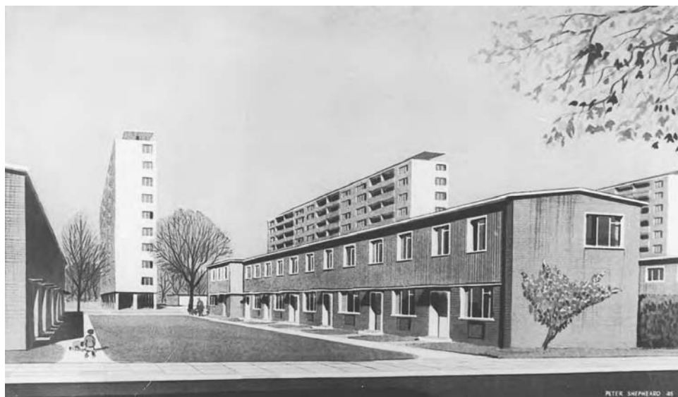
Figure 4.4 Mixed development of flats and housing in redevelopment areas became a new wartime model for site development, shown here in Greater London Plan proposals for West Ham. The flats were higher than any municipal blocks then existing. Both they and the (almost) flat-roofed long terraces built at right angles to the road show a strong continental modernist design influence.
