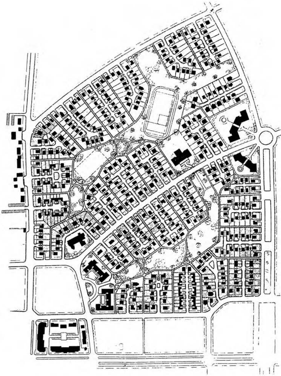
Figure 3.4 The other important American planning innovation of this period was the Radburn layout, perfected by Henry Wright and Clarence Stein. Heavily influenced by Perry's ideas, Radburn principles involved the separation of pedestrian and motor traffic, effectively updating the garden city vision for the motor age.
